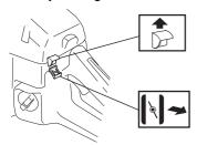
If the machine is fitted with a decompression valve (A): Press the valve to reduce the pressure in the cylinder and make starting easier. You should always use the decompression valve when starting the machine. Once the machine has started the valve will automatically return to its original setting.
