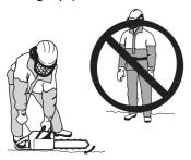
Place the chain saw on the ground and hold the rear handle down with your right foot. Grasp the front handle firmly using your left hand. Make sure the chain saw is steady and the chain is not touching the ground or other objects. Then grasp the starter handle with your right hand and pull the starter cord. Never wrap the starter cord around your hand
