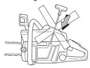
Pull the front hand guard towards the front handle. The chain brake is now disengaged. Your saw is ready for use.
