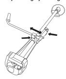
Now make a final adjustment, with the machine hanging from the harness, to obtain the most comfortable working position. Tighten the screws.
