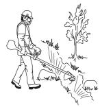
4 Switch off the engine before moving to another area. Fit the transport guard before carrying or transporting the equipment any distance.
