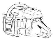
Clean the cooling system with a brush once a week, more often in demanding conditions. A dirty or blocked cooling system results in the machine overheating which causes damage to the piston and cylinder.
