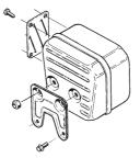
Some mufflers are equipped with a special spark arrestor mesh. If your machine has this type of muffler, you should clean the mesh at least once a week. This is best done with a wire brush.
