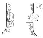
The directional cuts should run 1/4 of the diameter through the trunk and the angle between the top cut and bottom cut should be  $45^{\circ}$ .
