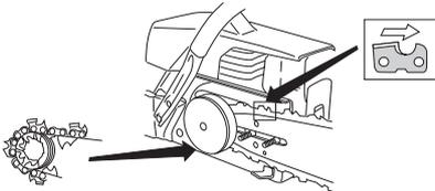
Make sure that the edges of the cutting links are facing forward on the top edge of the bar.
