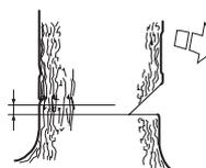
Set the spike bumper (if one is fitted) just behind the felling hinge. Use full throttle and advance the chain/bar slowly into the tree. Make sure the tree does not start to move in the opposite direction to your intended felling direction. Drive a wedge or breaking bar into the cut as soon as it is deep enough.
