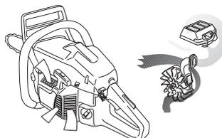
**IMPORTANT!** In order to maintain operation of the centrifugal cleaning system it must be regularly maintained.
