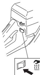
When the red mark on the switch is visible, the heating is on.
