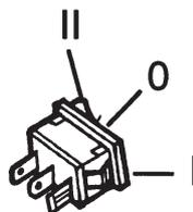
The switch is off in position "0", supplies current to the handle heater in position "I", supplies current to the carburettor in position "II".
