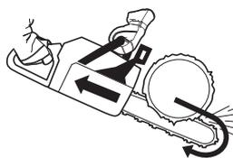
Unless the user resists this pushing force there is a risk that the chain saw will move so far backwards that only the kickback zone of the bar is in contact with the tree, which will lead to a kickback.
