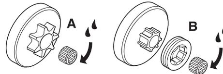
Both versions have a needle bearing on the drive shaft, which has to be greased regularly (once a week). CAUTION! Use a high-quality bearing grease or engine oil.
