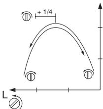
**CAUTION! If the chain rotates while idling the T-screw must be turned anti-clockwise until the chain stops.**
