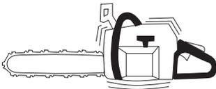
When you use a chain saw, vibration is generated by the uneven contact between the chain and the wood you are cutting.
