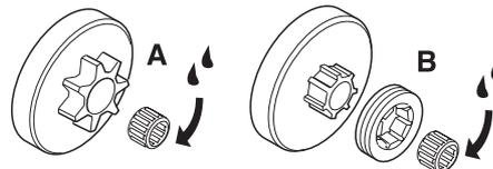
Both versions have a needle bearing on the drive shaft, which has to be greased regularly (once a week).
