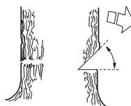
The line where the two cuts meet is called the directional cut line. This line should be perfectly horizontal and at right angles (90°) to the chosen felling direction.
