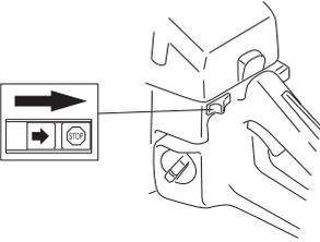
Stop the engine by switching off the ignition.
