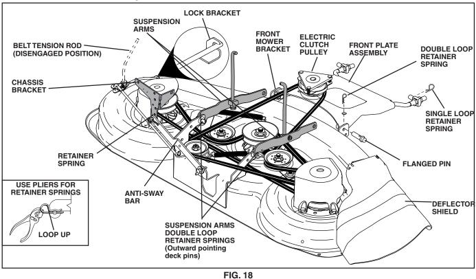
Position front plate assembly between front mower brackets. Raise deck and plate assembly to align holes and insert flanged pins. Secure pins with double loop retainer springs between the plate assembly and mower brackets.
