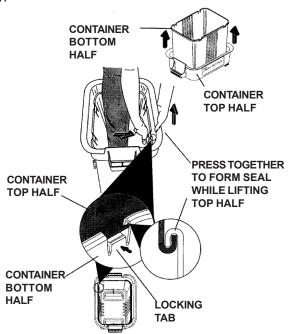
**ASSEMBLY CHECK:** Squeeze sides of lower half of container and check that there is no gap between upper and lower halves. If a gap appears, unlock tabs to separate container halves and repeat instructions above.
