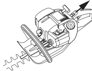
**Choke:** Set the choke control in the choke position. The choke position is also the automatic start throttle position.
