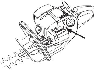
Hold the body of the machine on the ground using your left hand (CAUTION! Not with your foot!). Grip the starter handle, slowly pull out the cord with your right hand until you feel some resistance (the starter pawls grip), now quickly and powerfully pull the cord.
