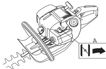
**Air purge:** Press the air purge diaphragm repeatedly until fuel begins to fill the diaphragm. The diaphragm need not be completely filled.
