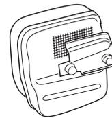
On mufflers without a catalytic converter the mesh should be cleaned weekly, or replaced if necessary. On mufflers fitted with a catalytic converter the mesh should be checked, and if necessary cleaned, monthly. **If the mesh is damaged it should be replaced.**
