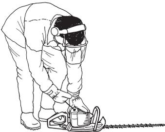
Push the choke control back to its original position as soon as the engine fires, and continue trying to start until the engine starts. When the engine starts, quickly apply full throttle to automatically disengage the start throttle setting.
