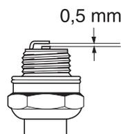
**CAUTION!** Always use the recommended spark plug type! Use of the wrong spark plug can damage the piston/cylinder.
