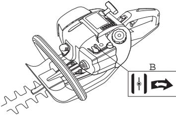
**Air purge:** Press the air purge diaphragm repeatedly until fuel begins to fill the diaphragm. The diaphragm need not be completely filled.
