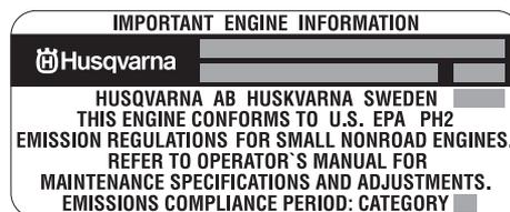
The Emissions Compliance Period referred to on the Emission Compliance label indicates the number of operating hours for which the engine has been shown to meet Federal emissions requirements. Category C = 50 hours, B = 125 hours, and A = 300 hours.
