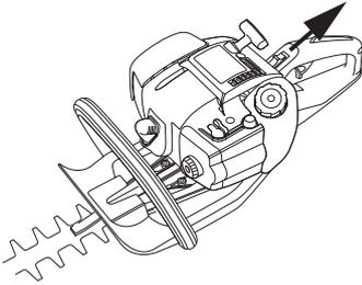
**Choke:** Set the choke control in the choke position and then back to its original position. This only engages the start throttle setting without any choke.
