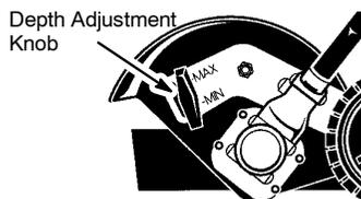
1. Loosen the depth adjustment knob.
