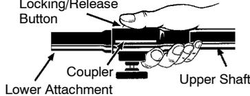
3. While securely holding the upper shaft, pull the attachment straight out of the coupler.
