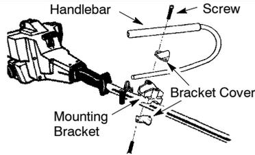
1. Place the mounting bracket over the upper shaft above the arrow on the safety label. Be sure to use the correct mounting bracket for either the 1" (2.5 cm) or 7/8" (2.2 cm) diameter upper shaft.
