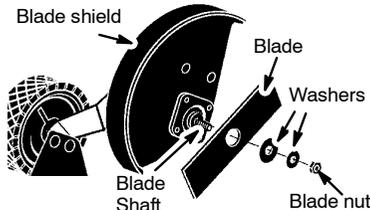
5. Install new blade onto blade shaft.
