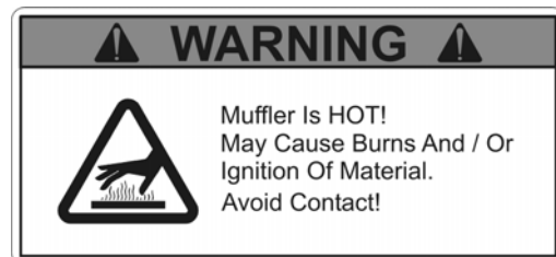
MUFFLER HOT, Front Side of Muffler Brace Right Side Top of Fan Shield 542 16 90-65* (x2)
