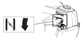
Hold the body of the machine on the ground using your left hand (CAUTION! Not with your foot!). Grip the starter handle, slowly pull out the cord with your right hand until you feel some resistance (the starter pawls grip), now quickly and powerfully pull the cord. **Never twist the starter cord around your hand.**
