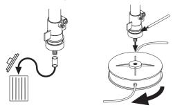
Screw the trimmer head onto the shaft.
