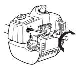
WARNING! If the idle speed cannot be adjusted so that the cutting attachment stops, contact your dealer/service workshop. Do not use the machine until it has been correctly adjusted or repaired.
