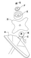
• Hook the blade guard/combination guard (A) onto the fitting on the shaft and secure with the bolt.
