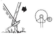
To fell a tree forwards, the bottom of the tree should be pulled backwards. Pull the blade backwards with a quick, firm movement.
