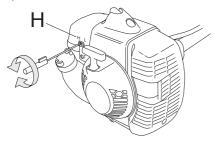
Note that the engine should be loaded when you adjust the high speed jet H. You should therefore fit the trimmer head T35 (2.7 mm cord) before adjusting the high speed jet. The cord length should be standard, i.e. to the knife on the trimmer guard.
