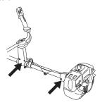
Using incorrectly wound cord or a blunt or incorrect cutting attachment (wrong type or incorrectly filed, see instructions under the heading Filing the blade) increases the level of vibration.
