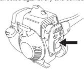
Some mufflers are equipped with a special spark arrestor mesh. If your machine has this type of muffler, you should clean the mesh at least once a week. This is best done with a wire brush. On mufflers without a catalytic converter the mesh should be cleaned weekly, or replaced if necessary. On mufflers fitted with a catalytic converter the mesh should be checked, and if necessary cleaned, monthly. If the mesh is damaged it should be replaced.
