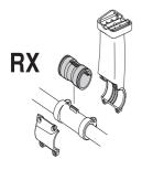
Check that the vibration damping element is undamaged and securely attached.
