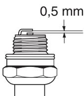
**CAUTION!** Always use the recommended spark plug type! Use of the wrong spark plug can damage the piston/cylinder. Check that the spark plug is fitted with a suppressor.
