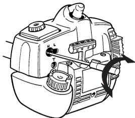
Apply full throttle and turn the high speed jet H very slowly clockwise until the engine slows down. Then turn the high speed jet H very slowly anticlockwise until the engine starts to run unevenly. Now turn the high speed jet H slowly clockwise a little way until the engine runs smoothly.
