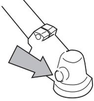
The grease in the bevel gear does not normally need to be changed except if repairs are carried out.
