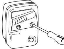
If the muffler on your machine is fitted with a spark arrestor mesh this must be cleaned regularly. A blocked mesh will cause the engine to overheat and may lead to serious damage.
