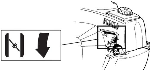
Hold the body of the machine on the ground using your left hand (CAUTION! Not with your foot!). Grip the starter handle, slowly pull out the cord with your right hand until you feel some resistance (the starter pawls grip), now quickly and powerfully pull the cord. **Never twist the starter cord around your hand.**
