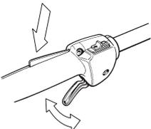
See instructions under the heading Start. Start the machine and apply full throttle. Release the throttle and check that the cutting attachment stops and remains at a standstill. If the cutting attachment rotates with the throttle in the idle position then the carburettor idle setting must be checked. See instructions under the heading Maintenance.
