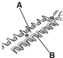
Check that the blade guard is not damaged or distorted. Replace the blade guard if it is bent or damaged.
