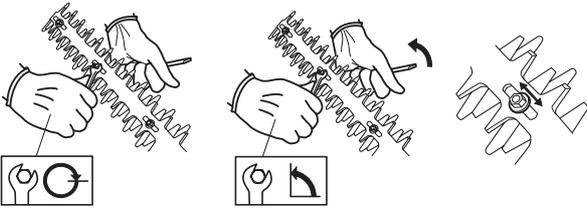
When the blades are correctly adjusted the play between the blades should be 0,2–0,4 mm, measured at the screws.
