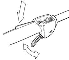
See instructions under the heading Start. Start the hedge trimmer and apply full throttle. Release the throttle trigger and check that the blades stop and remain stationary. If the blades move when the throttle trigger is in the idle position then the carburettor idle setting must be adjusted. See instructions under the heading Maintenance.
