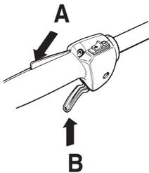
Make sure the throttle control is locked at the idle setting when the throttle lock is released.
