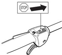
**CAUTION!** The stop switch automatically returns to the start position. In order to prevent unintentional starting, the spark plug cap must be removed from the spark plug when assembling, checking and/or performing maintenance.
