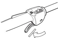
Press the throttle lock and make sure it returns to its original position when you release it.
