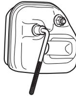
If the muffler on your machine is fitted with a spark arrester mesh this must be cleaned regularly. A blocked mesh will cause the engine to overheat and may lead to serious damage.
