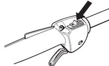
Start the engine and make sure the engine stops when you move the stop switch to the stop setting.
