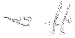
We recommend that you use a bar that is longer than the diameter of the tree, so that you can make the felling cut and directional cuts with single cutting strokes. See instructions under the heading Technical data section to find out which lengths of bar are recommended for your saw.
