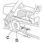
The front hand guard is not designed solely to activate the chain brake. Another important feature is that it reduces the risk of the chain hitting your left hand if you lose grip of the front handle.
