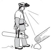
5 Take great care when cutting a tree that is in tension. A tree that is in tension may spring back to its normal position before or after being cut. If you position yourself
