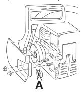
Fit the bar over the bar bolts. Place the bar in its rearmost position. Place the chain over the drive sprocket locate it in the groove on the bar. Begin on the top edge of the bar. Make sure that the edges of the cutting links are facing forward on the top edge of the bar.
