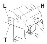
The L and H-jets are used to adjust the supply of fuel to match the rate that air is admitted, which is controlled with the throttle. If they are screwed clockwise the air/fuel ratio becomes leaner (less fuel) and if they are turned anticlockwise the ratio becomes richer (more fuel). A lean mixture gives a higher engine speed and a rich mixture gives a lower engine speed.
