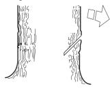
Next make the bottom cut so that it finishes exactly at the end of the top cut.
