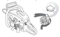
IMPORTANT! In order to maintain operation of the centrifugal cleaning system it must be regularly maintained. Clean the air intake to the starter, the fins on the flywheel, the space around the flywheel, inlet pipe and carburettor compartment.
