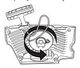
Undo the screw in the centre of the pulley and remove the pulley. Insert and fasten a new starter cord to the pulley.
