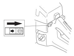
The engine is stopped by pushing the stop switch to the stop position.
