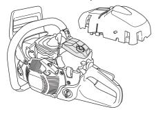
Remove the air filter after taking off the air filter cover.
