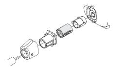
Regularly check the vibration damping units for cracks or deformation.
