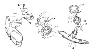
Fit the correct trimmer guard (A) for use with the trimmer head. CAUTION! Ensure that the guard extension is fitted.
