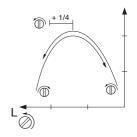
**CAUTION!** If the cutting attachment rotates when the engine is idling the idle adjustment screw T should be turned anticlockwise until the cutting attachment stops.
