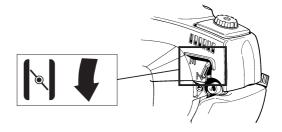
Hold the body of the machine on the ground using your left hand (CAUTION! Not with your foot!). Grip the starter handle, slowly pull out the cord with your right hand until you feel some resistance (the starter pawls grip), now quickly and powerfully pull the cord. **Never wrap the starter cord around your hand**
