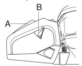
Make sure the throttle control is locked at the idle setting when the throttle lock is released.
