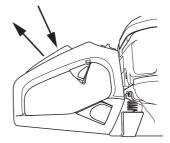
Check that the throttle control and throttle lock move freely and that the return springs work properly.
