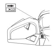
Start the engine and make sure the engine stops when you move the stop switch to the stop setting.
