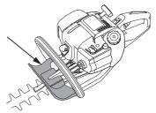
Check that the hand guard is fitted correctly. Check that the hand guard is undamaged.
