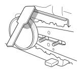
Regularly check that the brake band is at least 0.6 mm (0,024 inch) thick at its thinnest point.
