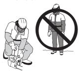
Always hold the saw with both hands. The right hand should be on the rear handle, and the left hand on the front handle. All people, whether right or left handed, should use this grip. Use a firm grip with thumbs and fingers encircling the chain saw handles.
