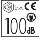
Noise emission to surroundings in accordance with the directive of the European Community. The machine's emission is indicated in the TECHNICAL DATA chapter and on the decal.
