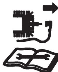
Switch off the engine and remove the ignition cable before carrying out repairs or maintenance
