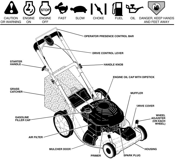
**IMPORTANT**: This lawn mower is shipped WITHOUT OIL OR GASOLINE in the engine.
