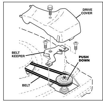
**FIG. 13** TO REPLACE DRIVE BELT (See Fig. 13)
