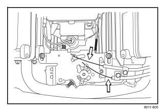
Throttle and choke cables by the carburetor
