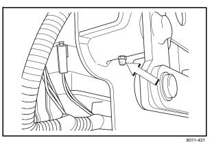
Lubricating the cutting height adjuster
