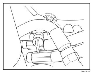
Fuel shut off valve, closed
