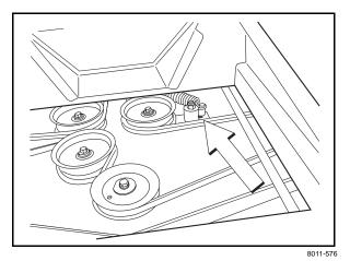
The belt adjuster grease zerk
