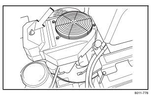
Remove the air filter cowling
