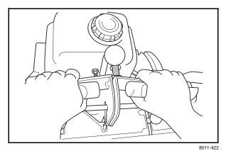
ETS-handle with motion control levers in reversing position
