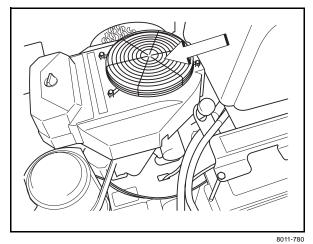
Check and clean the cooling air intake
