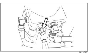
Vent screw on the hydraulic pump
