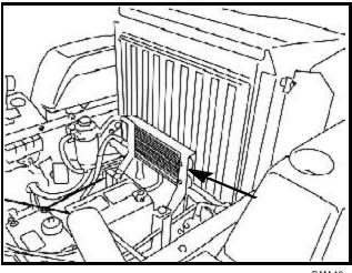
Check and clean the cooling air intake
