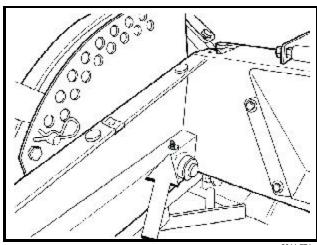
Lubricating the cutting height adjuster
