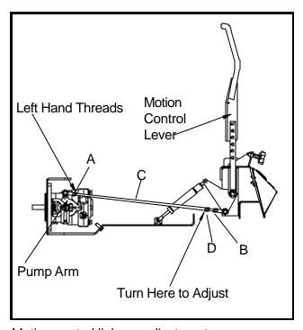
Motion control linkage adjustment
