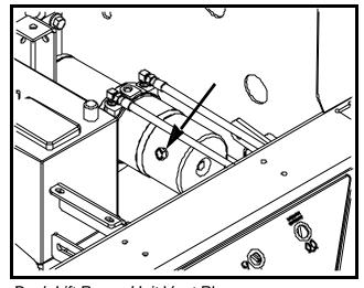
Deck Lift Power Unit Vent Plug
