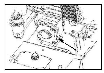
System relief valve on the hydraulic pump
