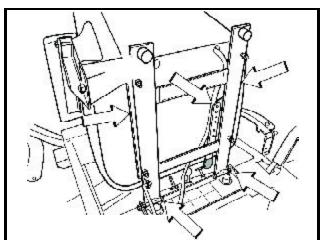
Lubricating the lengthways adjuster under the seat
