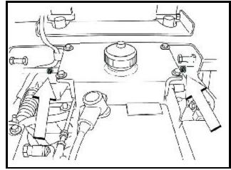
Lubricating the steering control shafts
