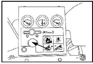
Disengaging the mower deck
