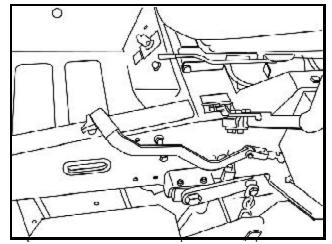
Parking brake in the disengaged position
