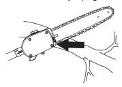
• Make an initial cut on the underside of the branch before cutting through the branch. This will prevent tearing of the bark, which could lead to slow healing and cause permanent damage to the tree. The cut should not be deeper than 1/3 of the branch thickness to prevent jamming. Keep the chain running while you withdraw the cutting attachment from the branch to prevent it jamming.
