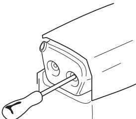
Some mufflers are equipped with a special spark arrestor mesh. If your machine has this type of muffler, you should clean the mesh at least once a week. This is best done with a wire brush. A blocked mesh will cause the engine to overheat and may lead to serious damage.
