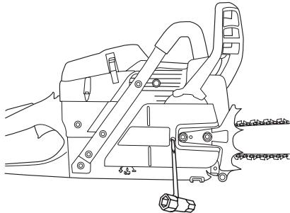
The chain is correctly tensioned when it does not sag from the underside of the bar, but can still be turned easily by hand. Hold up the bar tip and tighten the bar nuts with the combination spanner.
