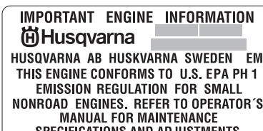
The Emissions Compliance Period referred to on the Emission Compliance label indicates the number of operating hours for which the engine has been shown to meet Federal emissions requirements. Category C = 50 hours, B = 125 hours, and A = 300 hours.
