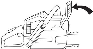
Remove the bar nuts and remove the clutch cover (chain brake). Take off the transportation ring (A).
