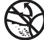
**WARNING!** Kickback may occur when the nose or tip of the guide bar touches an object, and cause a lightning fast reverse reaction, kicking the guide bar up and towards the operator. May cause serious personal injury.
