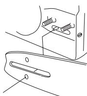
Tension the chain by turning the chain tensioning screw clockwise using the combination spanner. See instructions under the heading Tensioning the chain.
