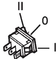
The switch is off in position "O", supplies current to the handle heater in position "I", supplies current to the carburettor in position "II".
