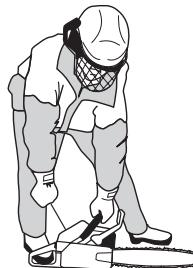
Push in the choke control as soon as the engine fire and make repeated starting attempts. Immediately press and release the throttle when the engine starts. That will disengage the throttle latch.
