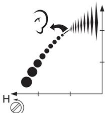
Note that the engine should not be under load when you adjust the high speed jet H. You should therefore remove the cutting attachment, nut, support flange and drive disc before adjusting the high speed jet H.
