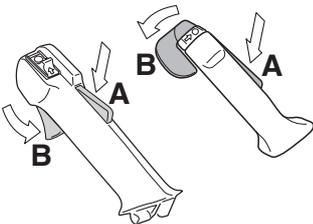
Make sure the throttle control is locked at the idle setting when the throttle lock is released.
