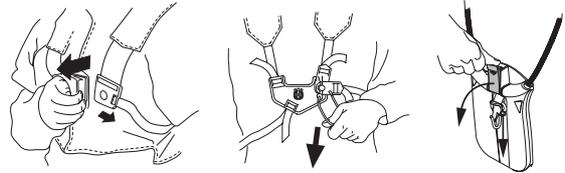
Check that the harness straps are correctly positioned. Once the harness and machine have been adjusted, check that the harness quick release works correctly.
