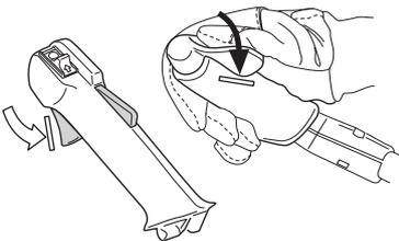
Press the throttle lock and make sure it returns to its original position when you release it.
