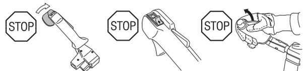
Start the engine and make sure the engine stops when you move the stop switch to the stop setting.
