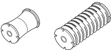
Regularly check the vibration damping units for cracks or deformation. Check that the vibration damping element is undamaged and securely attached.
