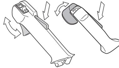
See instructions under the heading Start. Start the machine and apply full throttle. Release the throttle and check that the cutting attachment stops and remains at a standstill. If the cutting attachment rotates with the throttle in the idle position then the carburettor idle setting must be checked. See instructions under the heading Maintenance.
