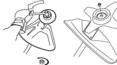
The nylon lining inside the locking nut must not be so worn that you can turn it by hand. The lining should offer a resistance of at least 1.5 Nm. The nut should be replaced after it has been put on approx. 10 times.
