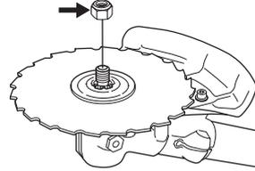
When fitting, tighten the nut in the opposite direction to the direction of rotation of the cutting attachment. To remove it, undo the nut in the same direction as the cutting attachment rotates. (CAUTION! The nut has a left-hand thread.)
