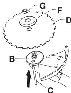
When loosening and tightening the saw blade nut, there is a risk of injury from the teeth of the saw blade. You should therefore always ensure that your hand is shielded by the blade guard when doing this. Always use a socket spanner with a shaft that is long enough to allow this. The arrow in the diagram shows the area where you should operate the socket spanner when loosening or tightening the nut.
