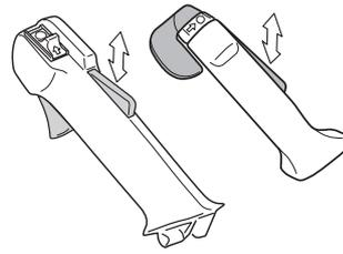
Check that the throttle control and throttle lock move freely and that the return springs work properly.
