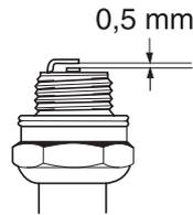
**CAUTION!** Always use the recommended spark plug type! Use of the wrong spark plug can damage the piston/cylinder. Check that the spark plug is fitted with a suppressor.
