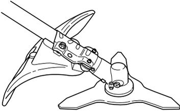
Check that the guard is undamaged and not cracked. Replace the guard if it has been exposed to impact or is cracked.
