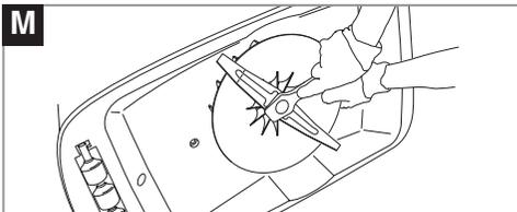
**Always handle the blade with care - sharp edges could cause injury. USE GLOVES. Never use more than 3 Cutting Height Spacers. Spacers must only be fitted between the blade and the fan and NEVER between the blade and the bolt.**
