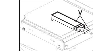
Install Rip Guide (V): Set Rip Guide (V) in desired position along Conveyor Cart (C) backstop. Tighten Knob to secure in position. Rip Guide (V) can be set to 90 degree position (as shown), or at 45 degrees to left or right.
