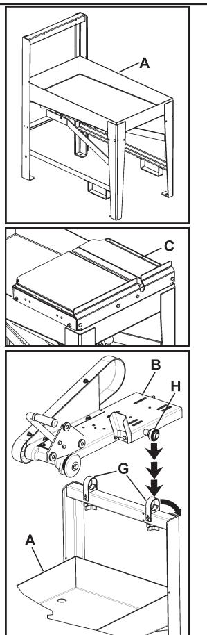
Pivot left and right Bearing Clamps (G) into their upper position. Tighten Knobs (K) until Bearing (H) of Head Platform (B) is secured into Pivot Block (J) of Pan Weldment (A).
