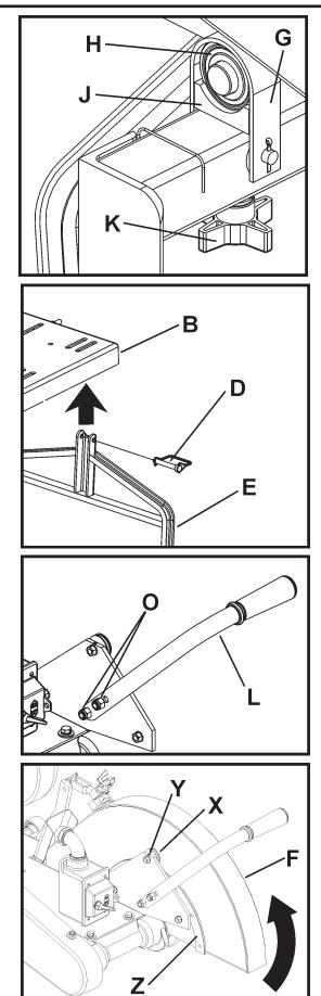
Install Tilt Arm (R) onto Blade Guard (F). Pivot Tilt Arm (R) upward until near Stud on Blade Guard (F). Pull collar on Tilt Arm (R) toward rear of machine, then connect with Stud on Blade Guard (F).
