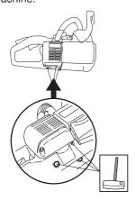
Some mufflers are equipped with a special spark arrestor mesh. If your machine has this type of muffler, you should clean the mesh at least once a week. This is best done with a wire brush. A blocked mesh will cause the engine to overheat and may lead to serious damage.
