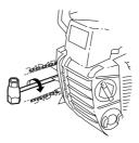
The chain is correctly tensioned when it does not sag from the underside of the bar, but can still be turned easily by hand. Hold up the bar tip and tighten the bar nuts with the combination spanner.
