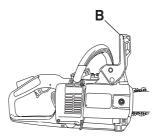
Move the front hand guard forwards and back to make sure it moves freely and that it is securely anchored to the clutch cover.
