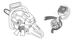
IMPORTANT! In order to maintain operation of the centrifugal cleaning system it must be regularly maintained. Clean the air intake to the starter, the fins on the flywheel, the space around the flywheel, inlet pipe and carburettor compartment.
