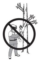
5 You must have a steady stance in order to have full control over the chain saw. Never work standing on a ladder, in a tree or where you do not have firm ground to stand on.
