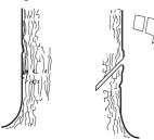
Next make the bottom cut so that it finishes exactly at the end of the top cut.
