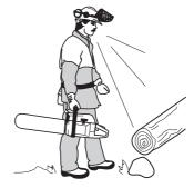
5 Take great care when cutting a tree that is in tension. A tree that is in tension may spring back to its normal position before or after being cut. If you position yourself incorrectly or make the cut in the wrong place the tree may hit you or the machine and cause you to lose control. Both situations can cause serious personal injury.
