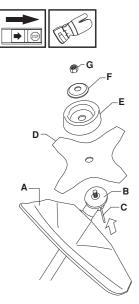
• Hook the blade guard/combination guard (A) onto the fitting on the shaft and secure with the bolt.
