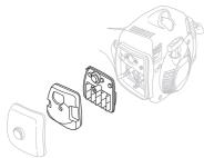
An oiled foam plastic filter (available as an accessory) must be used if the machine is operated in extremely dusty conditions. See instructions under the heading Oiling the air filter.
