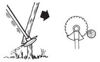
• To fell a tree forwards, the bottom of the tree should be pulled backwards. Pull the blade backwards with a quick, firm movement.
