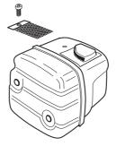
The muffler is designed to reduce the noise level and to direct the exhaust gases away from the operator. The exhaust gases are hot and can contain sparks, which may cause fire if directed against dry and combustible material.
