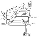
The chain is correctly tensioned when it does not sag from the underside of the bar, but can still be turned easily by hand. Hold up the bar tip and tighten the bar nuts with the combination spanner.
