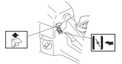
If the machine is fitted with an air purge (A): Press the air purge repeatedly until fuel begins to fill the bulb. The bulb need not be completely filled.
