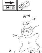
Hook the blade guard/combination guard (A) onto the fitting on the shaft and secure with the bolt.
