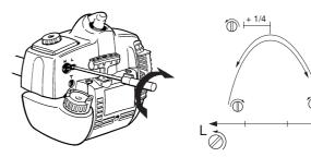
**CAUTION!** If the cutting attachment rotates when the engine is idling the idle adjustment screw T should be turned anticlockwise until the cutting attachment stops.
