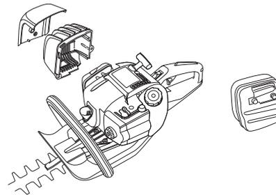
Some mufflers are equipped with a special spark arrester mesh. If your machine has this type of muffler, you should clean the mesh at least once a week. This is best done with a wire brush.
