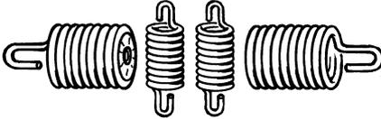
Regularly check the vibration damping units for cracks or deformation. Check that the vibration damping element is undamaged and securely attached.
