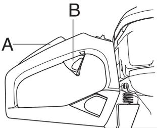
Make sure the throttle control is locked at the idle setting when the throttle lockout is released.
