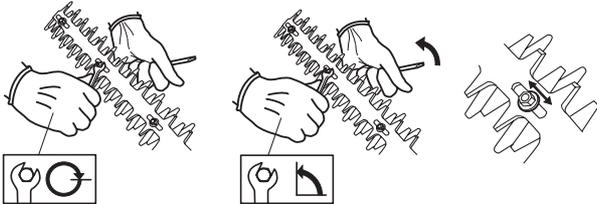
When the blades are correctly adjusted the play between the blades should be 0,2–0,4 mm, measured at the screws.
