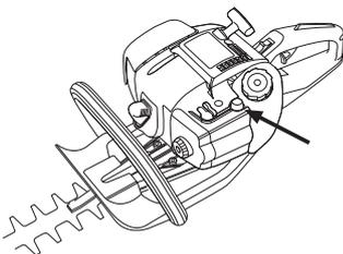
**Choke:** Set the choke control in the choke position.
