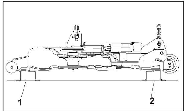
Adjust Deck Using Deck Leveling Blocks
