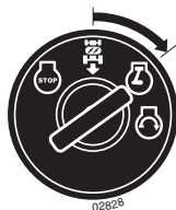
ENGINE "ON" POSITION (NORMAL OPERATING)
