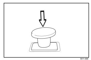
Depress the control for disengaging the mower deck
