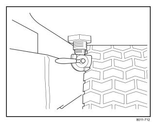
Fuel shut off valve in OFF position
