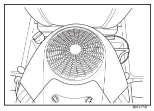
Check and clean the cooling air intake
