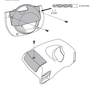
These reduce the cooling air and prevent large amounts of snow from being sucked into the engine.
