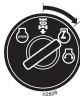
ENGINE "ON" POSITION (NORMAL OPERATING)
